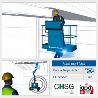
The unique pressure sensitive system acts as an 'emergency switch' in an entrapment situation. It is designed to react to the body pressure of an operator trapped against the boom lift's control panel.
