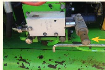
Hand Pump Manifold and Pump Handle Housing
