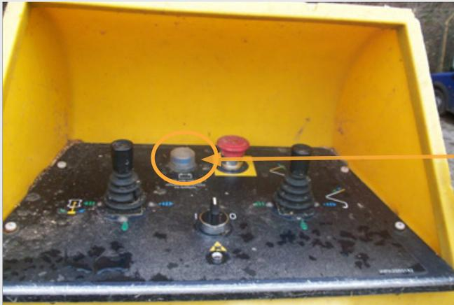
Emergency DC Power button press and hold to activate the electric motor.
