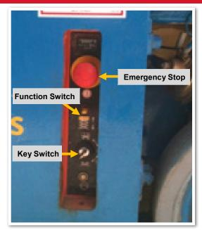
Machine shown is a 1932E3. Position of Emergency Handle and base controls may vary but controls on all have the same function.
